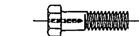
f. Bolt with cut threads and hole through head and unthreaded shank.
